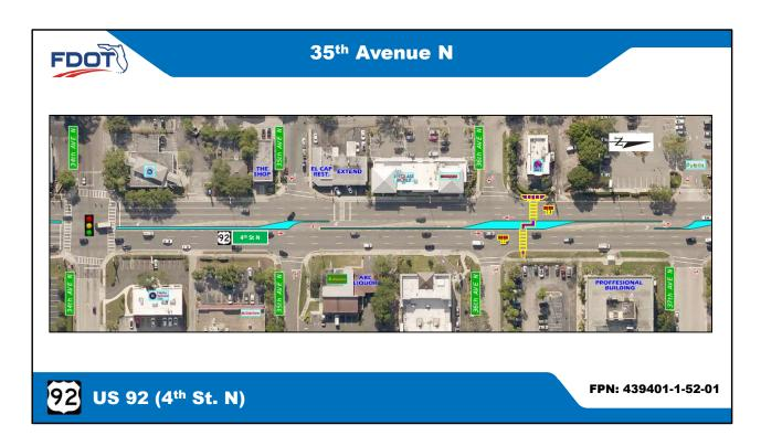
A raised median will be constructed at 35<sup>th</sup> Ave N to only allow right turns onto 4<sup>th</sup> St. N.
