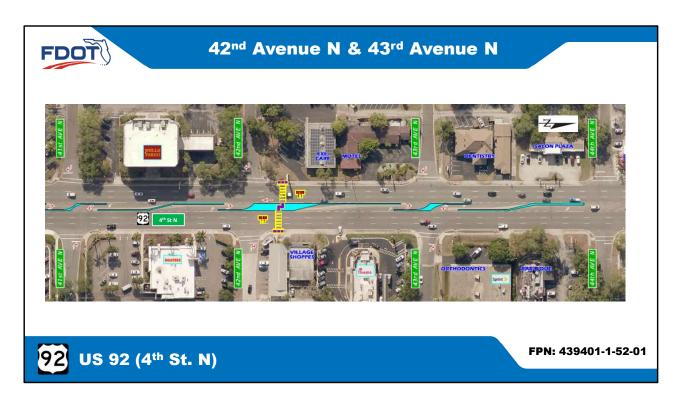
A raised median will be constructed at 42<sup>nd</sup> Ave N and 43<sup>rd</sup> Ave N to only allow right turns onto 4<sup>th</sup> St. N.
