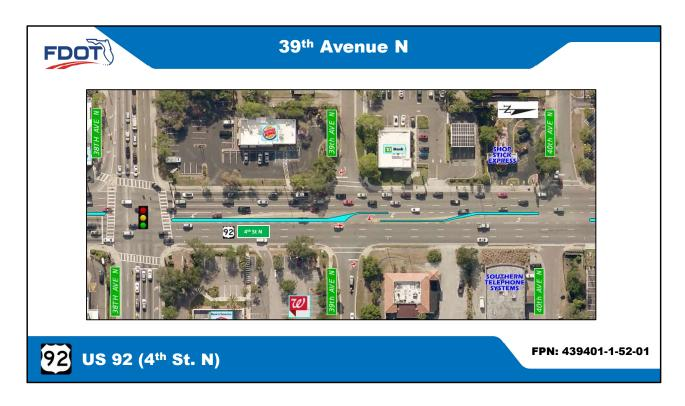
A raised median will be constructed at 39th Ave. N. to only allow right turns onto US 92 (4th St. N.) This modification is implemented to lengthen the left turn lane from southbound 4<sup>th</sup> St. to 38<sup>th</sup> Avenue N. for additional vehicle storage.
