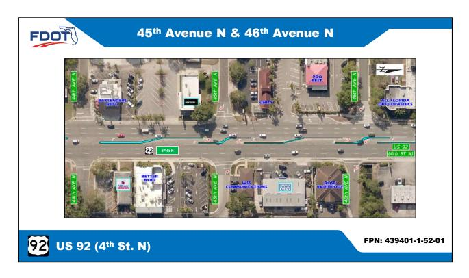
A raised median will be constructed at  $45^{th}$  Ave N and  $46^{th}$  Ave N to only allow right turns onto  $4^{th}$  St. N.
