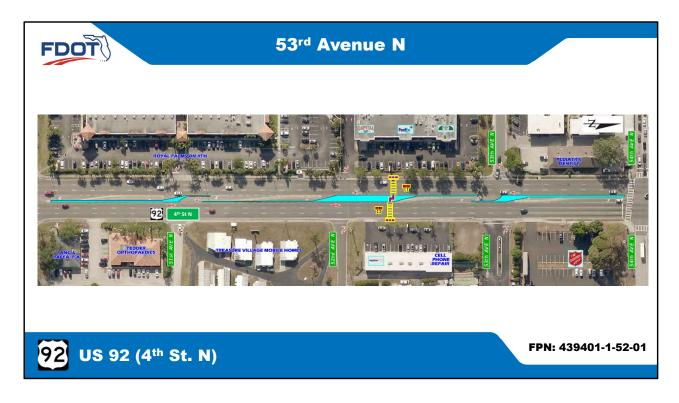
The median at 53<sup>rd</sup> Ave. N. will be modified to only allow right turns onto 4<sup>th</sup> St N.
