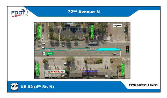
A raised median will be constructed at  $72^{nd}$  Ave N to only allow right turns onto US 92 (4<sup>th</sup> St. N).
