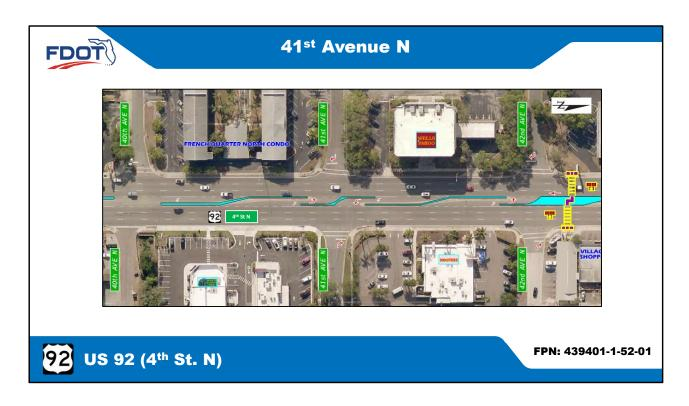
The median at 41st Avenue N. will be modified to only allow only allow right turns onto US 92 (4th St. N).
