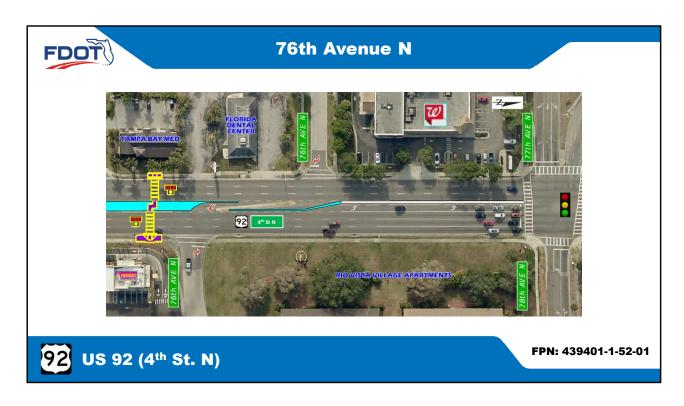
A raised median will be constructed at 76<sup>th</sup> Ave N to only allow right turns onto 4<sup>th</sup> St.
