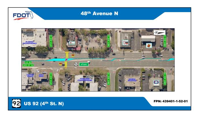
A raised median will be constructed  $48^{th}$  Ave N to only allow right turns onto  $4^{th}$  St. N.
