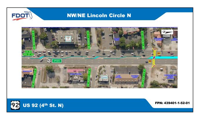
A raised median will be constructed at NW/NE Lincoln Circle to only allow right turns onto US 92 (4<sup>th</sup> St. N).
