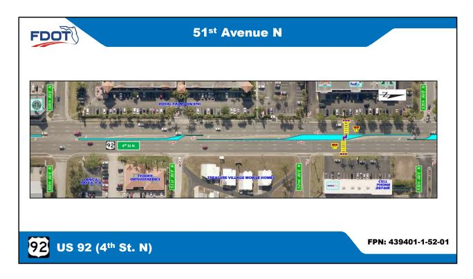
A raised median will be constructed at 51st Ave N to only allow right turns onto US 92 (4th St. N).
