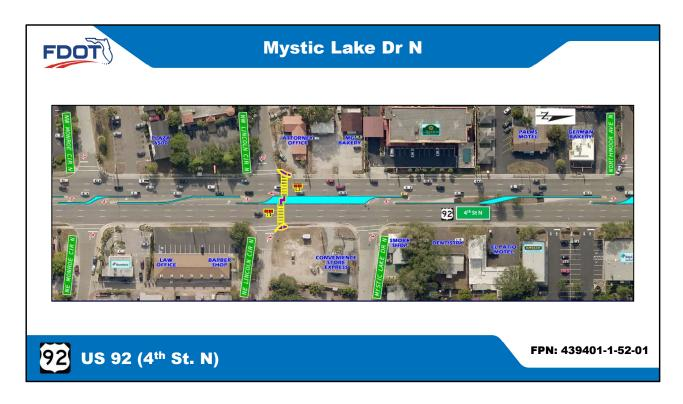
A raised median will be constructed at Mystic Lake Dr N to only allow right turns onto  $4^{\text{th}}$  St. N.
