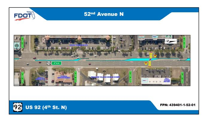
The median at  $52^{nd}$  Avenue N. will be closed to only allow right turns onto US 92 (4th St. N.).
