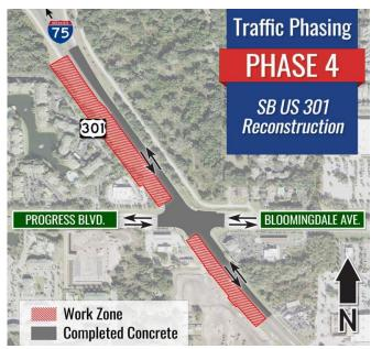
The Florida Department of Transportation is replacing the asphalt pavement with a durable concrete surface at the intersection of US 301 and Progress Boulevard/Bloomingdale Avenue and repaving US 301 between Lake St. Charles Boulevard and Progress Boulevard/Bloomingdale Avenue in Hillsborough County.
