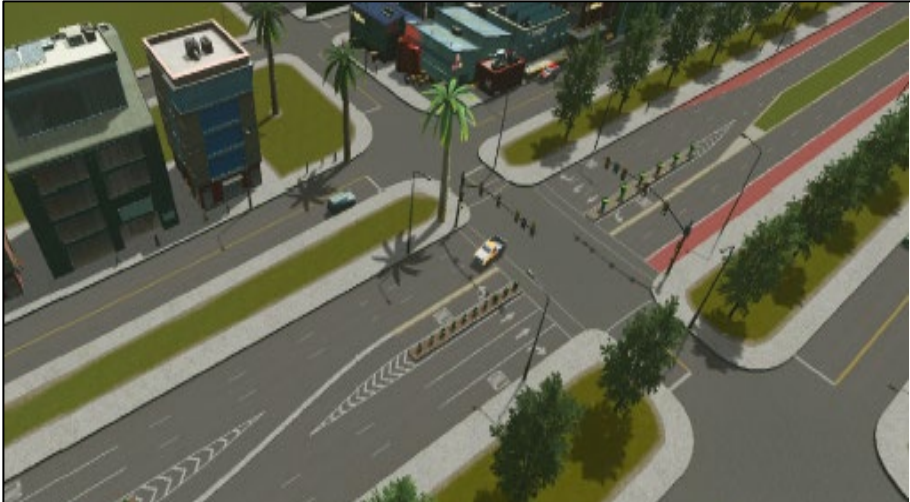
Intersection with Positive Offset Turn Lane Suggested to be Considered at E. 21 st Avenue.
